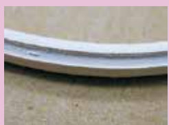
Incumbent Material after 20,000 wafer counts
