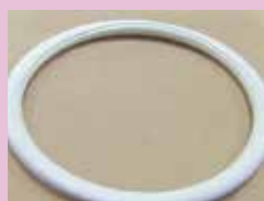
Incumbent Material after 20,000 wafer counts
